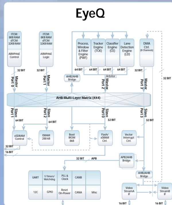
Figure 1. EyeQ Block Diagram
