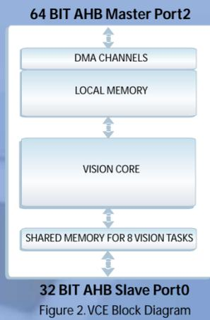
Figure 2. VCE Block Diagram
